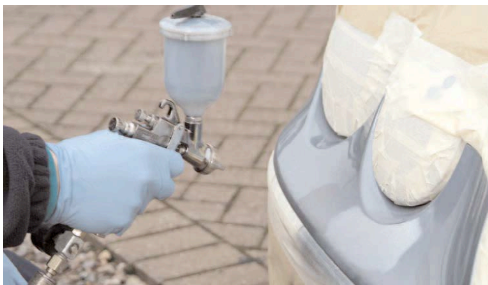
Figure 2 Typical SMART repair
